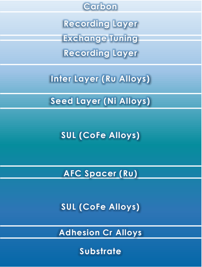
Layers layout of HDD
